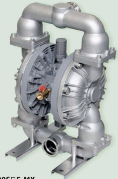
D500S□F-MX FDA Type Electro Polished SUS Pump. 2½" Sanitary Flange Connections. 520 L/min Max Flow Rate. (PTFE Diaphragms) 8mm Max Solids Size.
